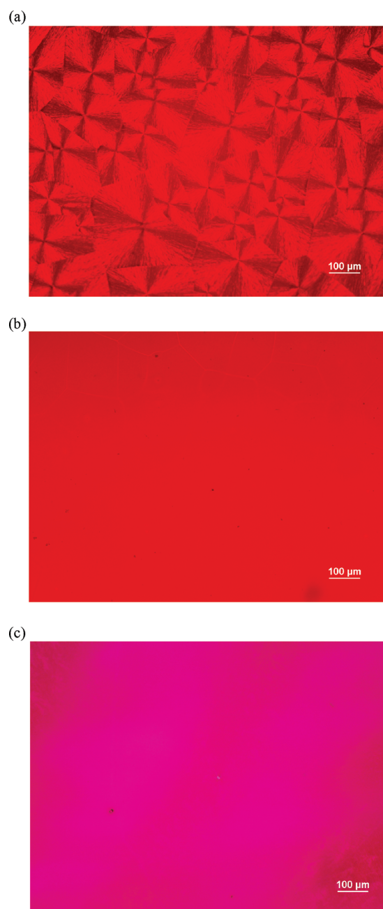
Figure 6. Polarized optical microscopy images (a, c) and fluorescence optical microscopy image (b) of a binary blend of PEO- b -P(nBMA- r -PgMA) and Rhodamine B azide before (a, b) and after (c) annealing at 110 °C for 12 h. The mole ratio between the alkyne groups and azide groups was 1:1.
